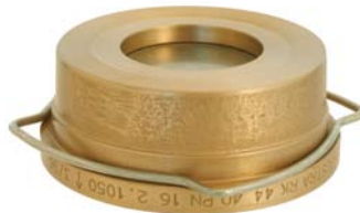
RK 44 with spiral centering PN 6 to PN 16, body material bronze, valve disc of austenitic steel
